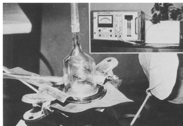
Modified leaf chamber to measure the rate of CO 2 exchange in upper and lower leaf sides. Inset shows the complete experimental set-up.
